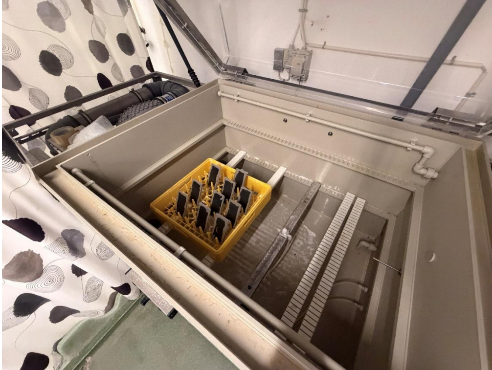
Photo 2 Test set-up salt mist. Before exposure.
